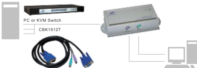
Connection of Transmitter
